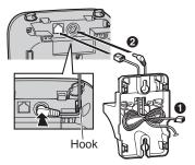
Insert the hooks on the wall mounting adaptor into holes ♠ and
